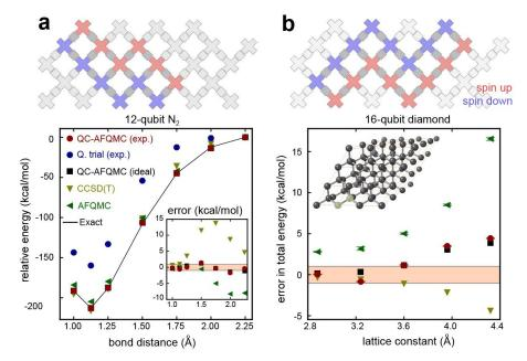
The energies from the Monte Carlo calculation driven by the quantum trial wavefunction are **highly accurate** (red circles) even though the bare trial wavefunction is not (blue circles)
