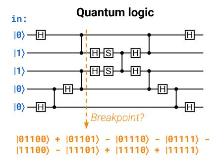
**Linear superposition** in high-dimensional space Measurement **collapses** to one bitstring
