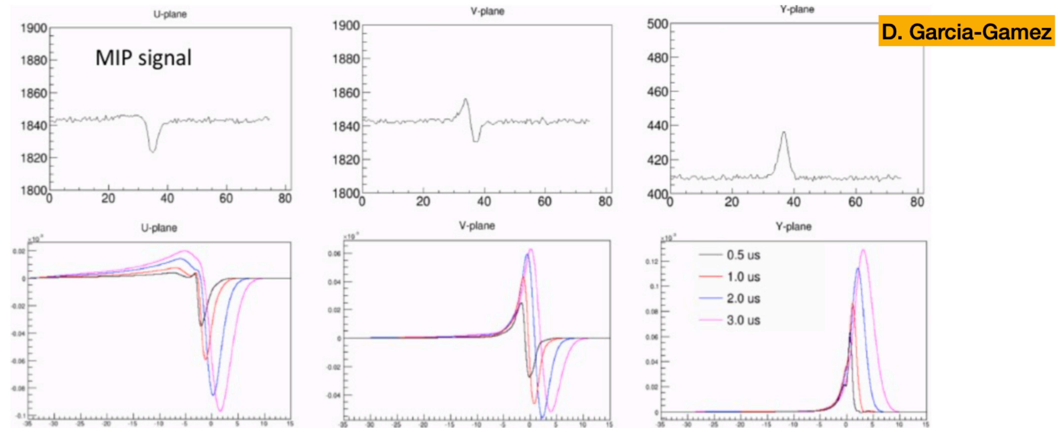
Digitised signal after the ADC = ionisation signal convoluted with the detector and electronics response functions then digitised at a fixed frequency
