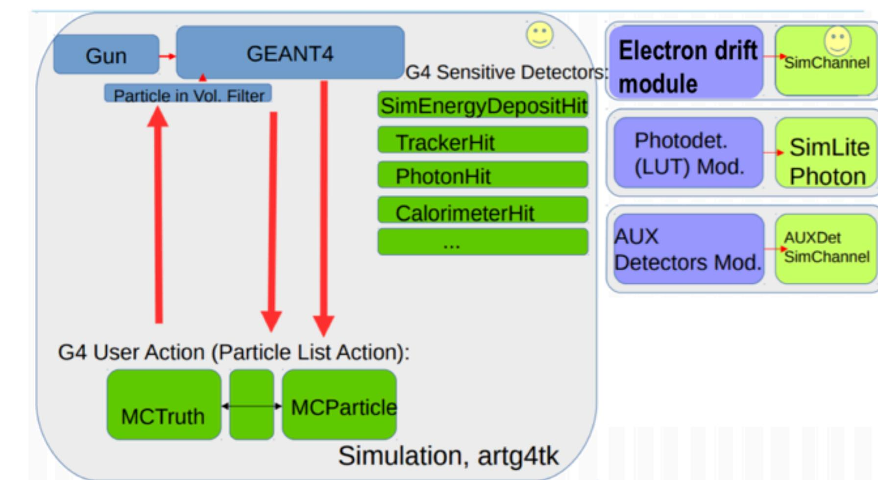
Only simulate particle interaction; separate plugin modules for electron drift, scintillation photons and auxiliary detectors
