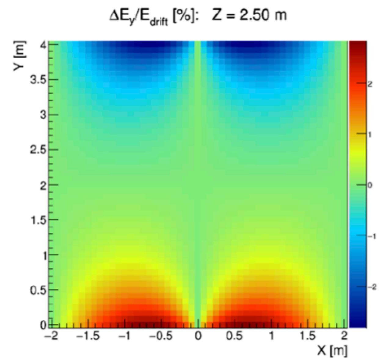
Corrections due to field distortions (space charge effect) are applied
