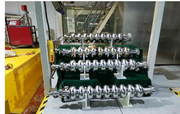
1.3 GHz High Q Mid-T Cavity Horizontal Test
