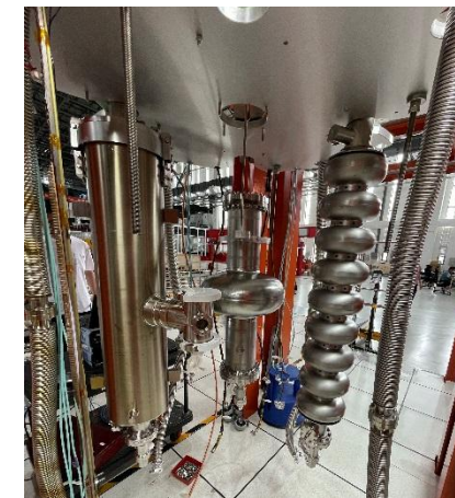
Vertical test of SRF cavities
