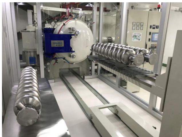
Vacuum furnace: Nitrogen doping, annealing, baking
