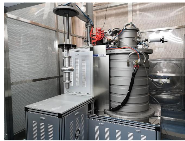
Furnace for Nb 3 Sn coating
