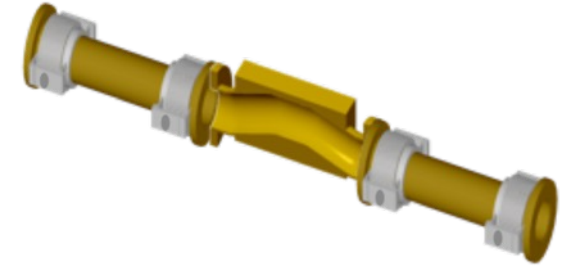
KEKB type collimator in the arc-sections
