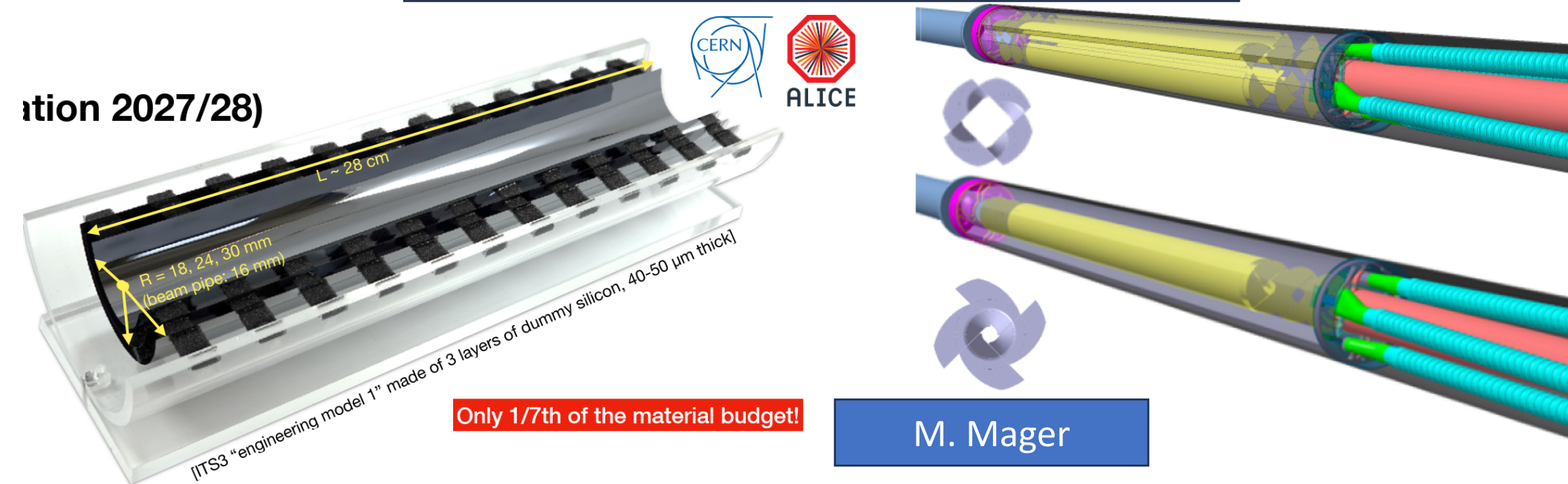
Curved detector for HL-LHC upgrades
