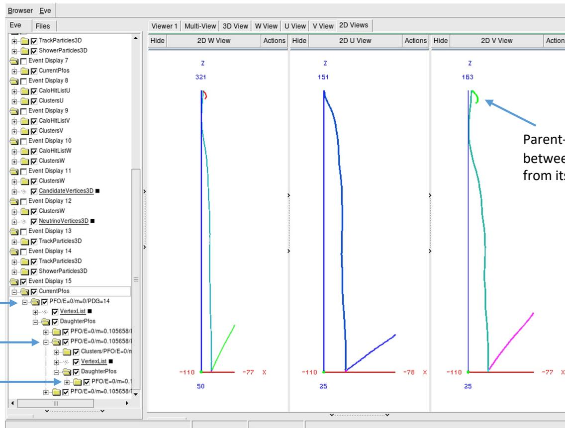
Parent-daughter link is made between muon and the particle from its secondary interaction
