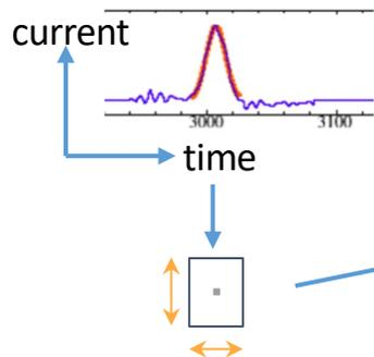
The X-width of the hit is from the Gaussian fit to the waveform, and the Z-width is the wire-spacing distance
