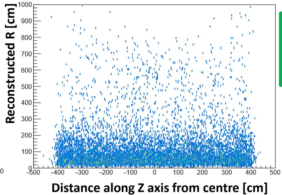
No correlation between the reconstructed values and the position of the capture
