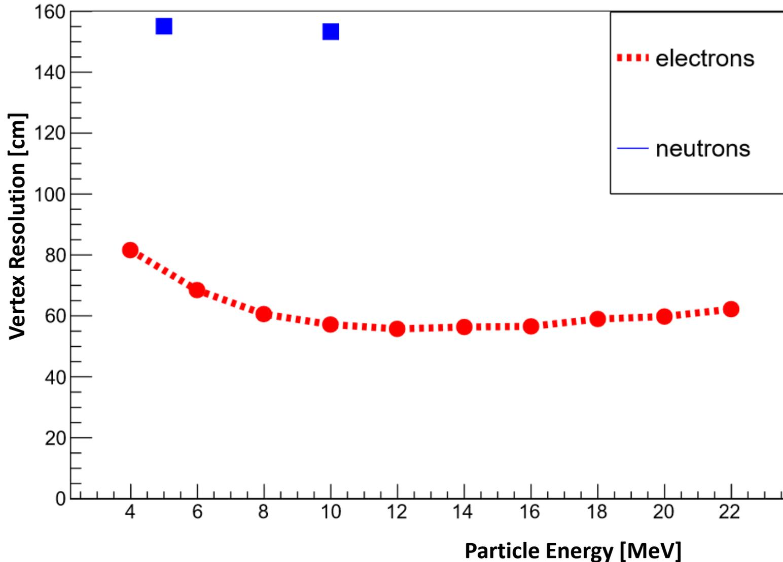
Neutron vertex resolution worse than electron vertex resolution.
