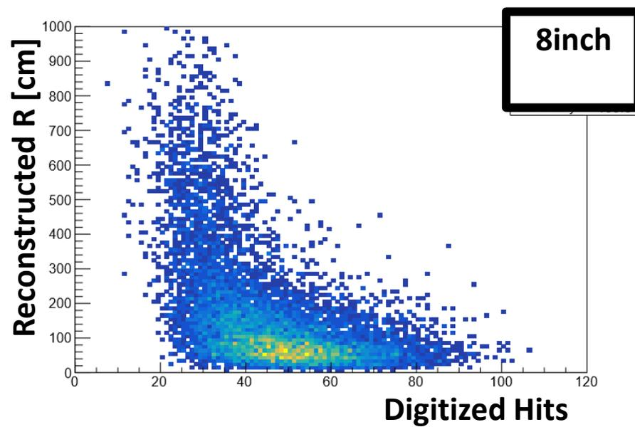
3" PMT configuration shows many events with less than 20 hits, whereas 8" configuration rarely has less than 20 hits.
