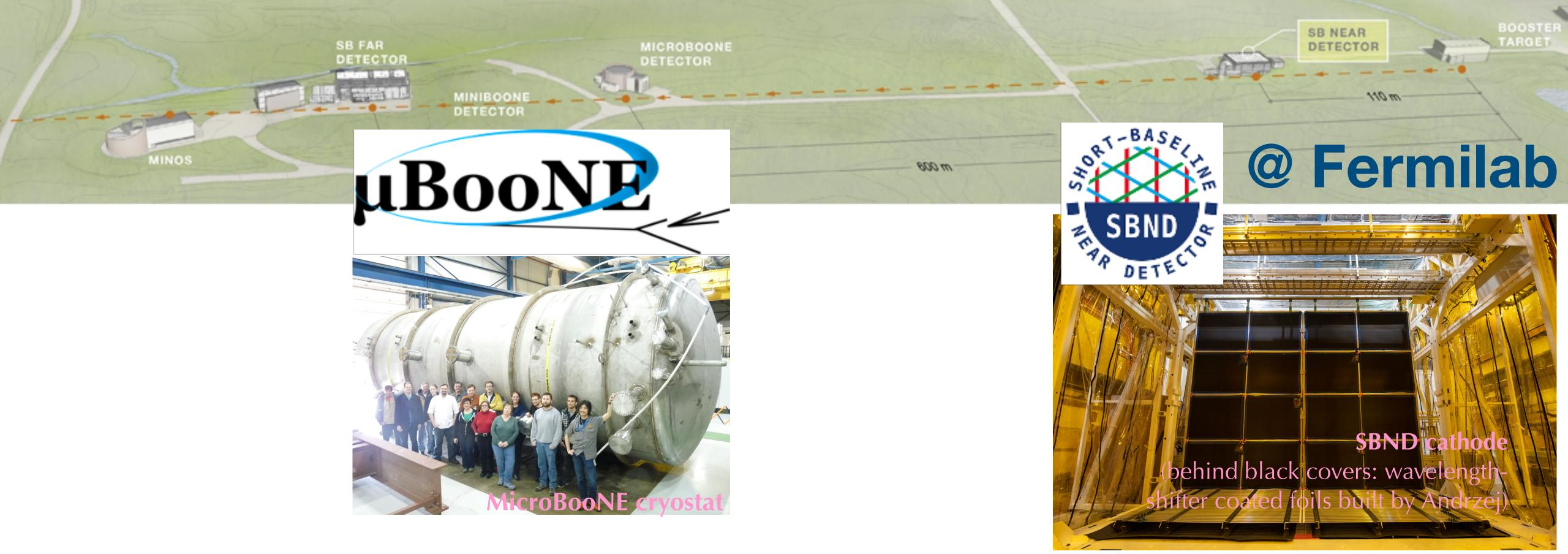
Short-baseline neutrino experiments:  $\nu_{\mu}$ ,  $(\bar{\nu}_{\mu})$  beam created at target →Liquid Argon (LAr) detectors at **110m** and **470m**  $\blacksquare$  Look for  $\nu_e(\bar{\nu}_e)$  appearance,  $\nu_\mu(\bar{\nu}_\mu)$  disappearance for new, sterile, neutrino(s).
