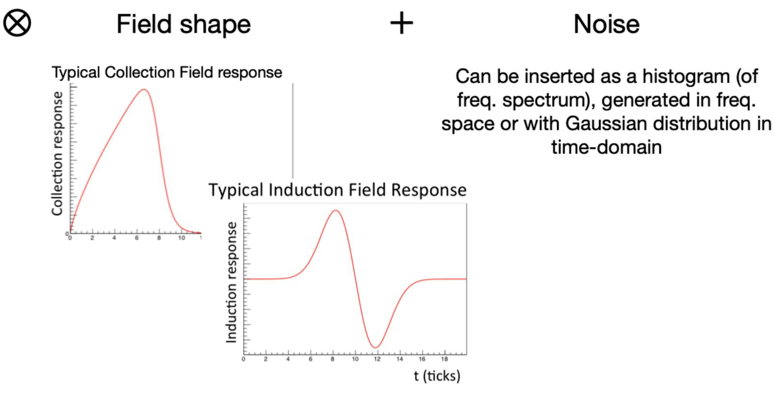
Response to channels to drifting electrons as a function of time
