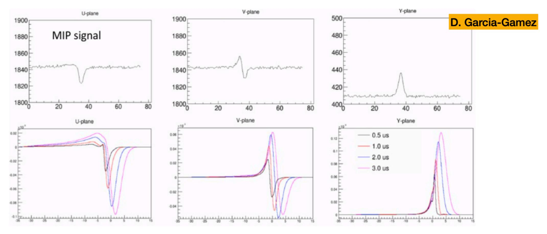
Digitised signal after the ADC = ionisation signal convoluted with the detector and electronics response functions then digitised at a fixed frequency
