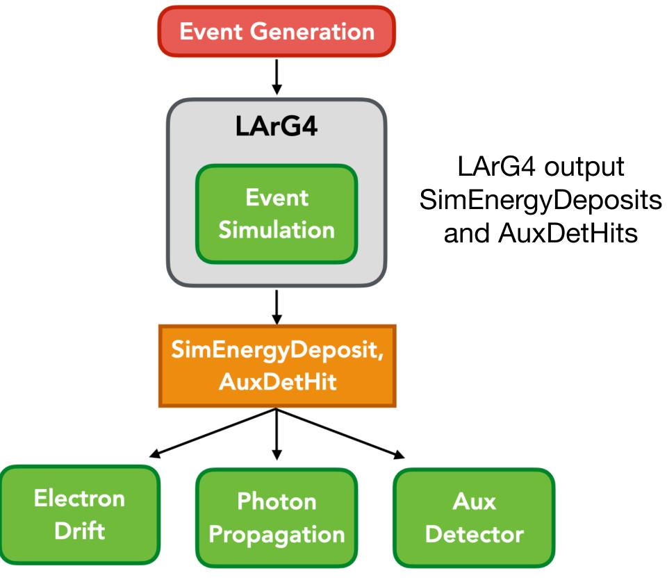
Ionisation, electron drift, optical simulation, CRT simulation is done by different LArSoft modules
