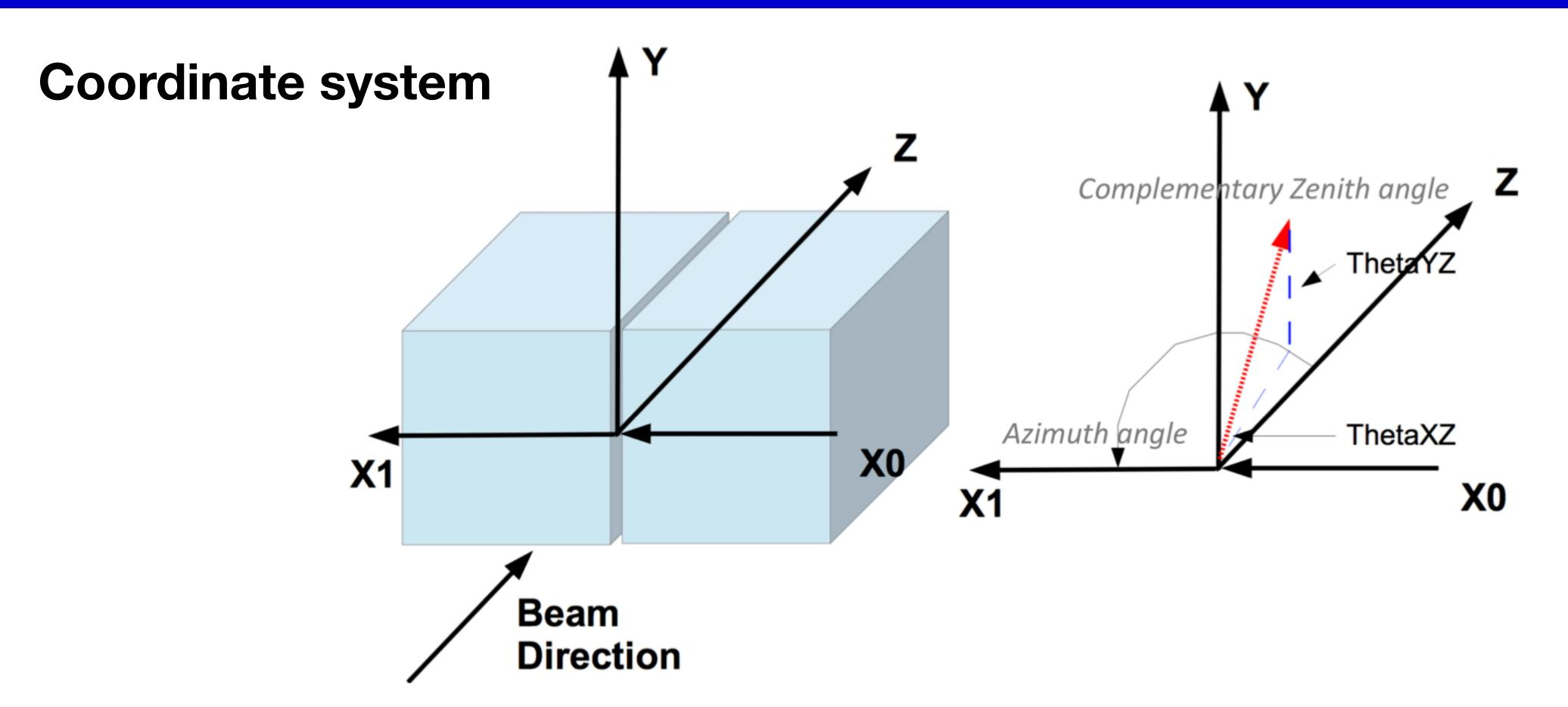
For all detectors: Z increases in the direction of neutrino travel, Y increases away from the centre of the Earth and X increases so as to make a right-handed coordinate system.
