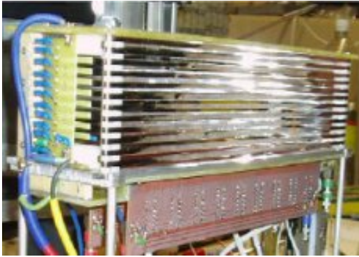
Time Projection Chambers (TPCs) at F2 and F4 measure the position .
