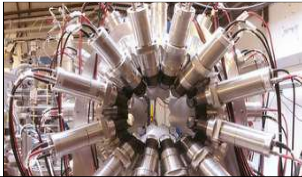
Fast TIMing Array \text{LaBr}_3(\text{Ce}) modules ( FATIMA )
