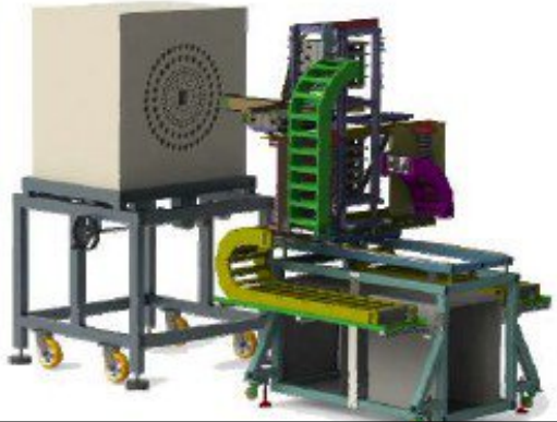
BEta-deLAYed Neutron detector ( BELEN ) 48 ^3\text{He} cylindrical counters
