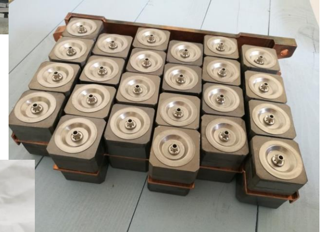
Boron carbide (B 4 C) validated by ITER as a shielding material for diagnostics.
