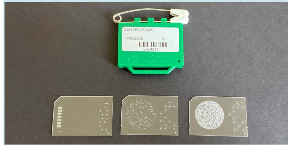
PADC dosemeter top, PADC plastic below, before and after processing
