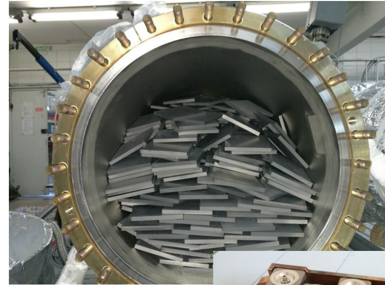
Boron carbide (B 4 C) validated by ITER as a shielding material for diagnostics.
