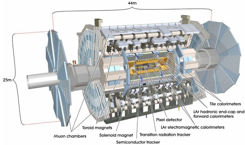
ATLAS Detector 140M Readout channels
