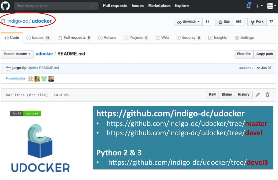
udocker is a basic user tool to execute simple docker containers in user space without requiring root privileges. Enables download and execution of docker containers by non-privileged users in Linux systems where docker is not available. It can be used to pull and execute docker containers in Linux batch systems and interactive clusters that are managed by other entities such as grid infrastructures or externally managed batch or interactive systems.
